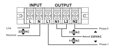
Connection for single output: 110VAC or 115VAC or 120VAC
