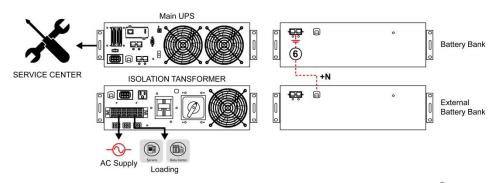
Step 3: When UPS is returned from repair service, please connect cable ①, cable ②, cable ③, cable ④, cable ⑤ of step 1. Make sure all cables are firmly connected, and then turn on the input breaker of mains and change over the maintenance bypass switch from "MAINT." to "INV.", lastly , lastly press "ON" button to turn on the UPS.
