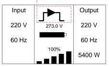
The LCD display in bypass mode without output is shown in the following.
