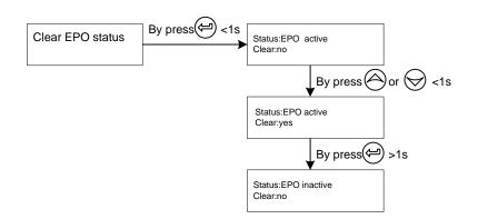
Note: First make sure the EPO signal is inactive or the LCD will show below information and the EPO active status couldn't be cleared.
