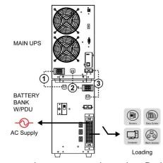
Step 2: Main UPS box can be sent to repair service. During UPS maintenance, you can connect UPS AC input connection cable to UPS AC output connector, refer to below cable ①. Turn on input breaker of mains to supply power to loadings.
