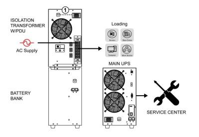
Step 3: When UPS is returned from repair service, please connect cable ①, cable ③ of step 1. Make sure all cables are firmly connected.
