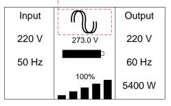
The function could be enabled through the LCD setting or the software, Winpower. The load should be derated to 60% in converter mode.
