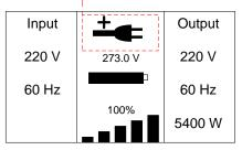
The function could be enabled through the LCD setting or the software, Winpower. It is attention that the transfer time of UPS output from HE mode to battery mode is about 10ms. But it is still too long for some sensitive load.
