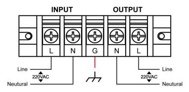
(2) Input: 1P2W+G, 220/230/240VAC ; Output: 1P3W+G, 110/220VAC or 115/230VAC or 120/240VAC
