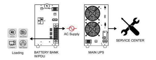
Step 3: When UPS is returned from repair service, please connect cable ①, cable ③ of step 1. Make sure all cables are firmly connected.
