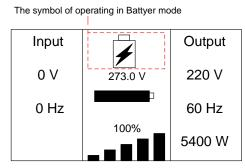
When the UPS is running in battery mode, the buzzer beeps once every 4 seconds.
