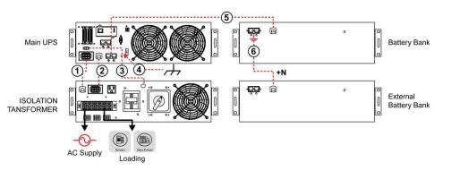
Step 2: Main UPS box can be sent to repair service. The load connected on Isolation Transformer box will continuously be supplied by AC mains.
