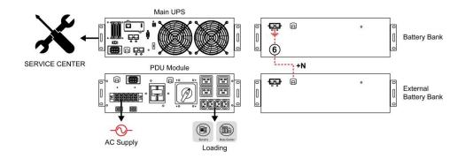
Step 3: When UPS is returned from repair service, please connect cable ①, cable ②, cable ③, cable ④, cable ⑤ of step 1. Make sure all cables are firmly connected, and then turn on the input breaker of mains and change over the maintenance bypass switch from "MAINT." to "INV.", lastly press "ON" button to turn on the UPS.
