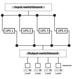
9) Do not switch on the output breaker of each UPS, switch on the input breaker of the each UPS, the UPS should work in bypass with output, observe their display to check if there are any warning or fault information, measure the output voltage of each UPS separately to check if the voltage difference between them is less than 1V. If the difference is more than 1V, check the wiring.
