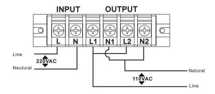
Note: Please make sure that the input and output wires and the input and output terminals are connected tightly.
