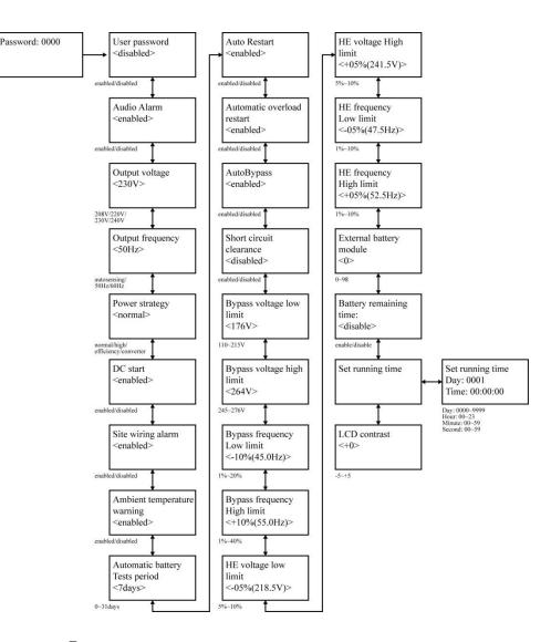
By press on the menu of "Identification", the display would enter the next setting menu tree if "User password" is disabled. If "User password" is enabled, the user should enter the password by press , , , and , then enter the next setting menu tree.
